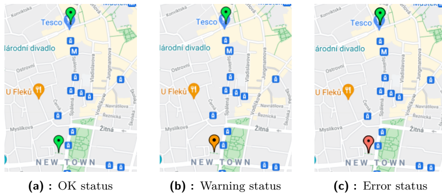
Figure 3.30: Device states on the map: Sufficient battery voltage and data are sent properly (a). Low device battery voltage (b). The device is completely discharged or there is no signal at all (c).
